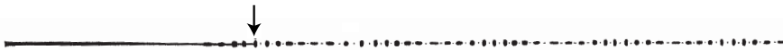
Figure 1.1: A figure from Savart's original paper of 1833 is reproduced here. 1,2 This sketch depicts the spontaneous breakup of a 6 mm diameter water jet into droplets. The time scale on which the breakup takes place is very short \tau_{\text{cap}} \approx 20 ms. The arrow indicates the location of droplet pinch-off.
